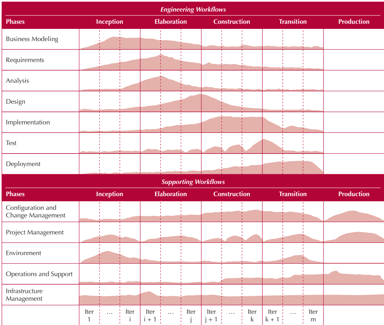
FIGURE 2-9 The Enhanced Unified Process
